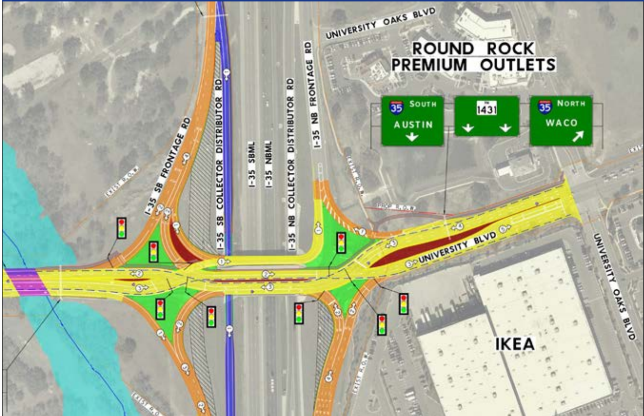
Figure 14: TxDOT is using a Diverging Diamond Intersection to improve traffic flow in Round Rock
