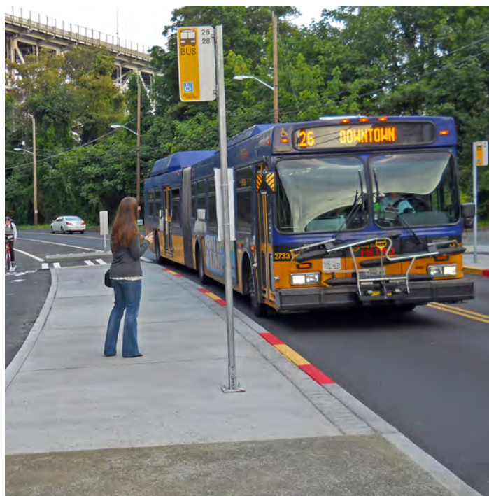
Floating transit stop in Seattle gives separation for buses and bicyclists and provides refuge for transit riders to wait
