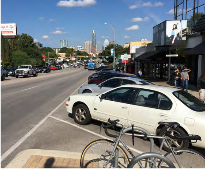
Head-out angled parking provides direct sight lines for motorists to see other vehicles and bicyclists
