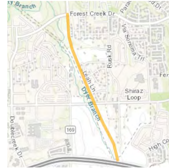
Kenney Fort Blvd, Seg. 2.3 Construct limited access six-lane divided major arterial roadway. City of Round Rock / Williamson County $12,250,000 / CORR2RD
