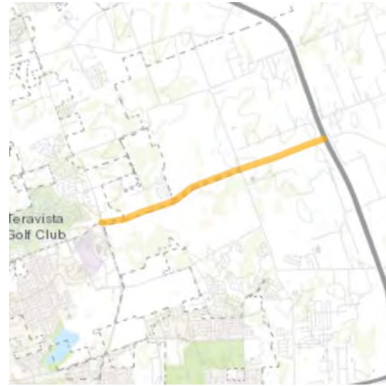
University Blvd. Reconstruct to four-lane divided roadway. City of Round Rock/ Williamson County, Construction $6,300,000 / CORR1RD
