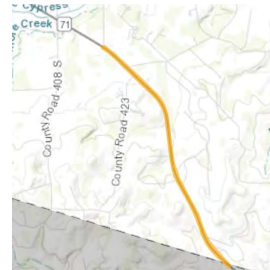
SH 71 Reconstruct to four 12-foot lanes, 14-foot continuous turn lane and 10-foot shoulders. Burnet County / TxDOT $9,720,000 / BUC20RD
