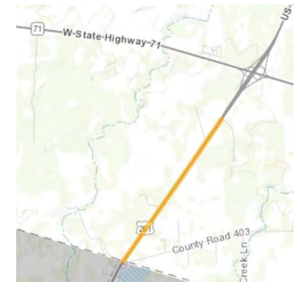
US 281 Reconstruct to four 12-foot lanes, 14-foot continuous turn lane and 10-foot shoulders. Burnet County / TxDOT, Construction $5,616,000 / BUC14RD
