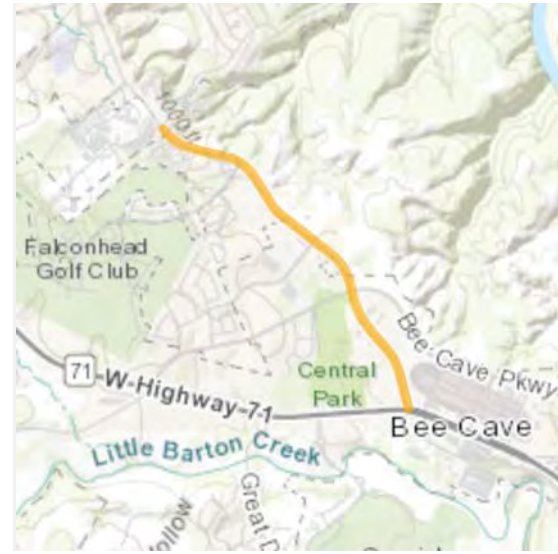
RM 620 Upgrade from four-lane to six-lane divided. TxDOT / City of Lakeway, Construction $18,000,000 / TxD16RD
