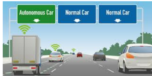
Dedicated CAV lane
