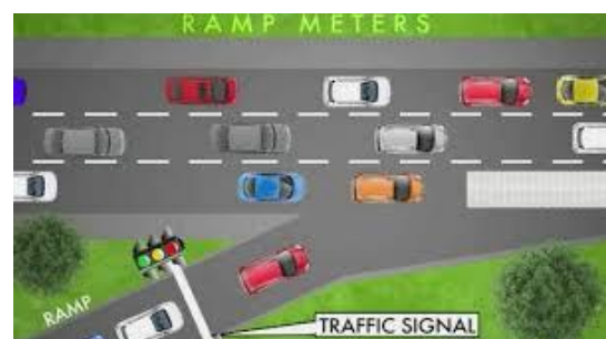
Ramp Metering design
