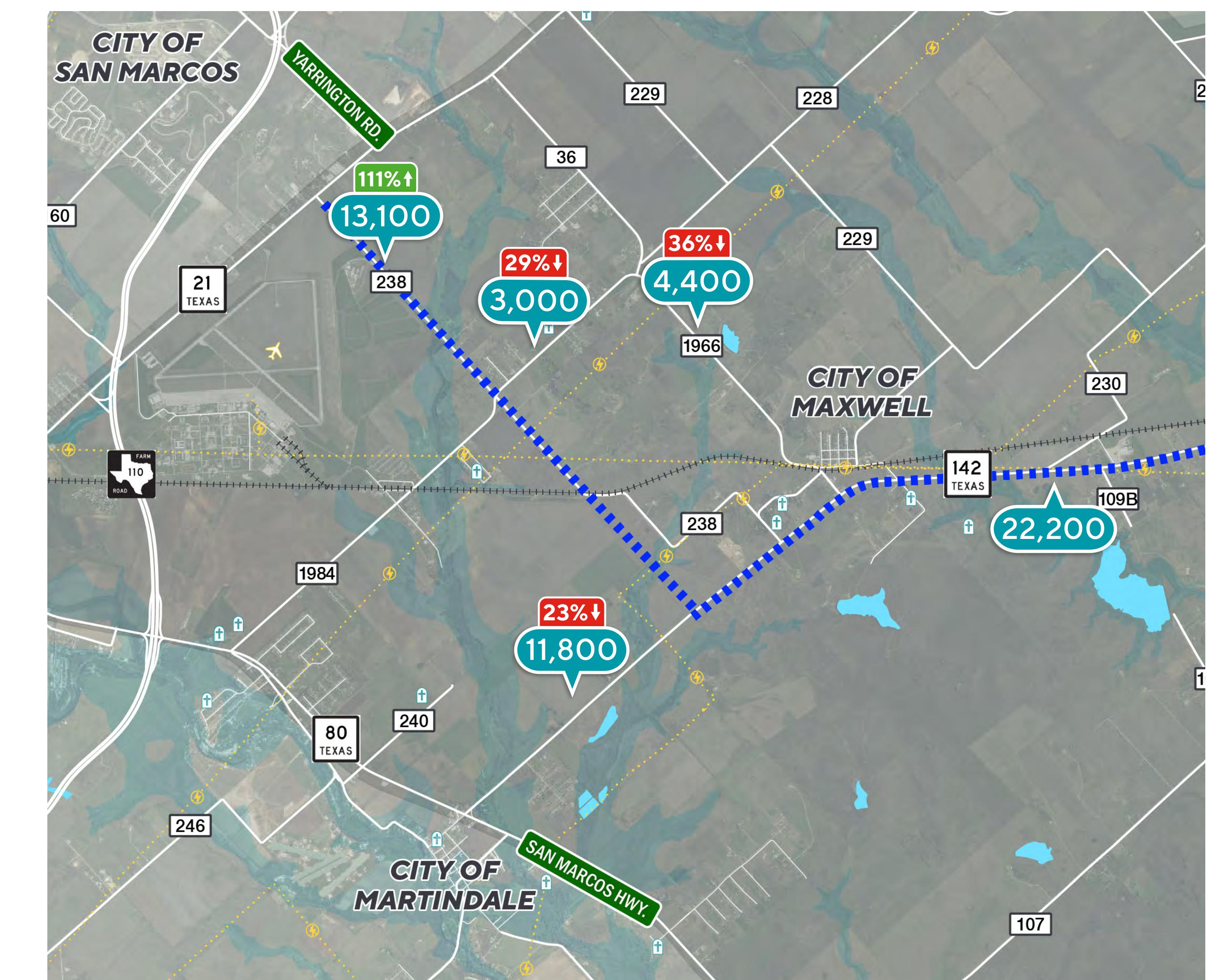
Average daily traffic reflects the projected traffic volume per day on each roadway in the study area. With the blue and green routes in combination, traffic is distributed across multiple east-west routes in the network and provides options to drivers for destinations to the northwest and southwest.
