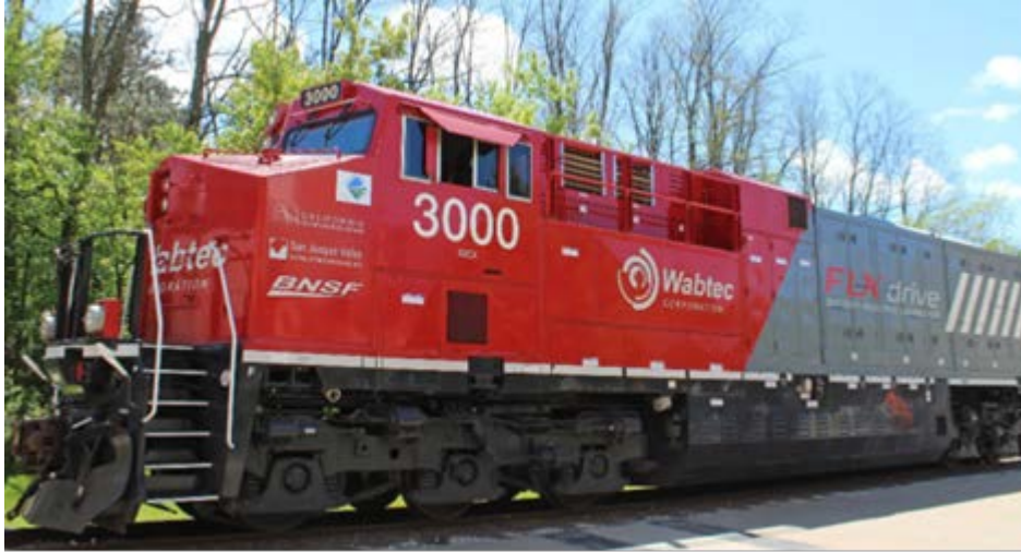
Figure 24: Wabtec FLXdrive Battery-Electric Locomotive
