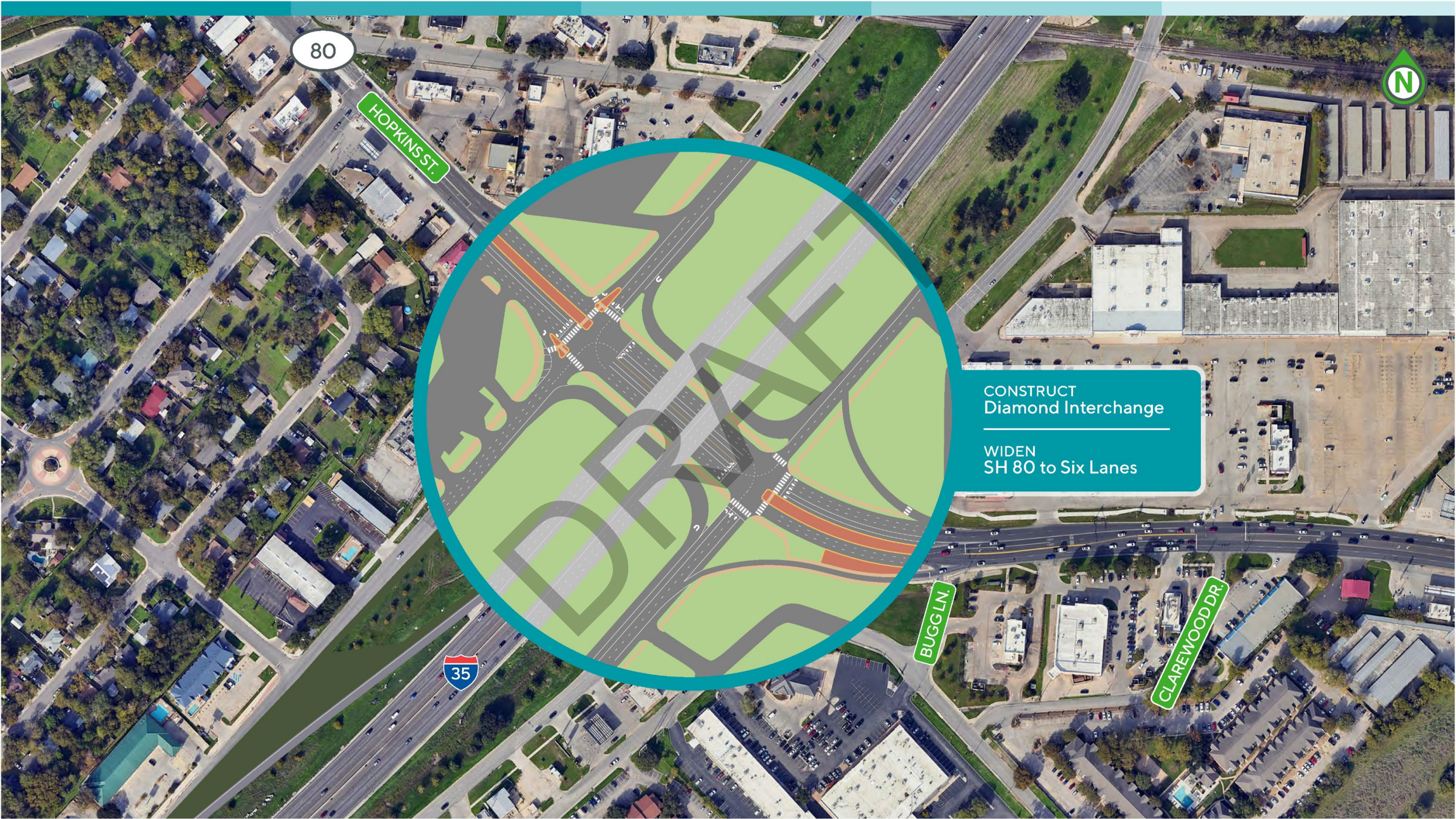
Figure 14: Long-Term Intersection Improvements: IH-35 / SH 80
